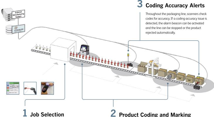
The product or appropriate code can be selected at the CLARiSUITE™-installed PC or Videojet printer. Or, a bar code can be scanned from a work order or from the product itself with a hand-scanner.
